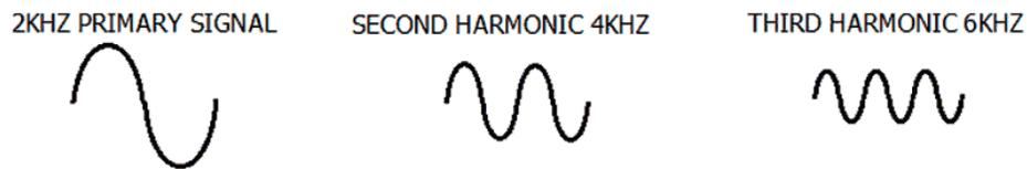
Generally speaking, the higher harmonic frequencies are lower in amplitude. By the time you get to the eighth or ninth harmonic the harmonics may be too low to measure. This only applies to sine waves; square wave harmonics are significantly higher.
